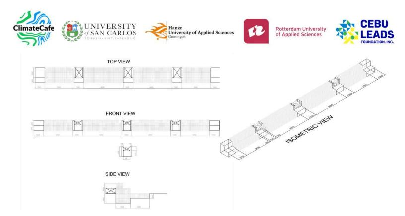
*Figure 5. CAD Generated Plan of the Check Dam (Scaled)*
